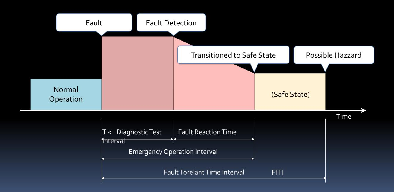
Fault reaction time and fault tolerant time interval (ISO26262-1 Fig.4)
